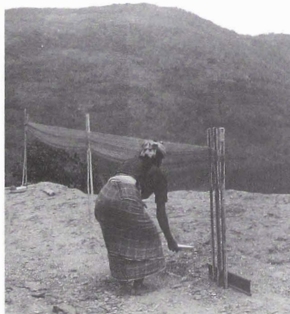
Above Heddle-making for a diamond pattern. Picking up the heddle loops for the second heddle between pick-up stick A and cross stick 2.
