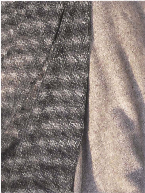
The soft, natural-coloured, pashmina shawls on the right are woven on 4-shaft frame looms in Kathmandu, usually with a cotton warp and pashmina weft in a 2/2 twill weave. The shawl on the left is the first trial (in 1992) by a dhaka weaver from east Nepal using pashmina weft on a black cotton warp with natural colour silk and black cotton inlay patterns.
