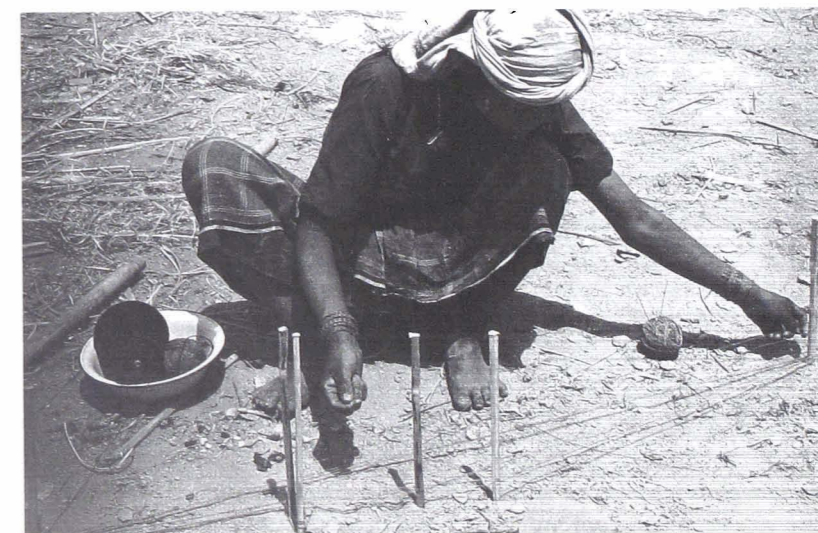
Right Forming heddle loops during warping over the pair of sticks on the left.
